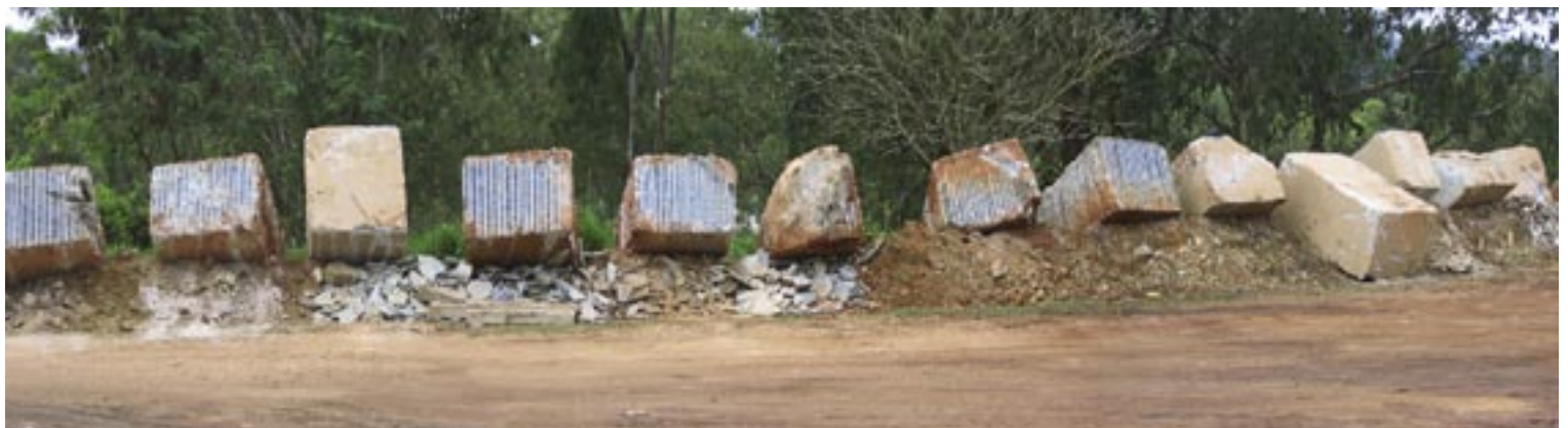
Soapstone blocks ready for milling
