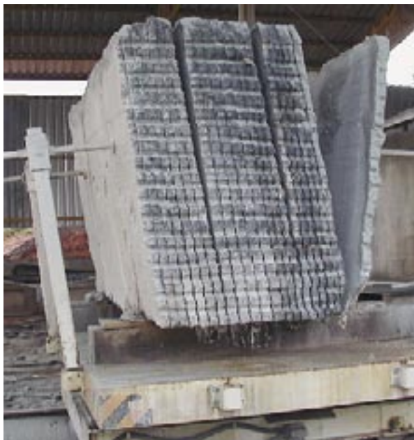
The system of block cutting ensures even thickness
