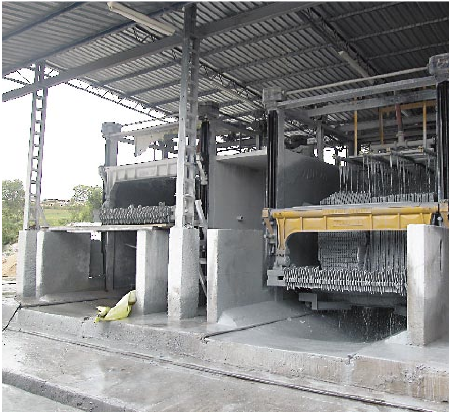
Blocks are cut into plates
