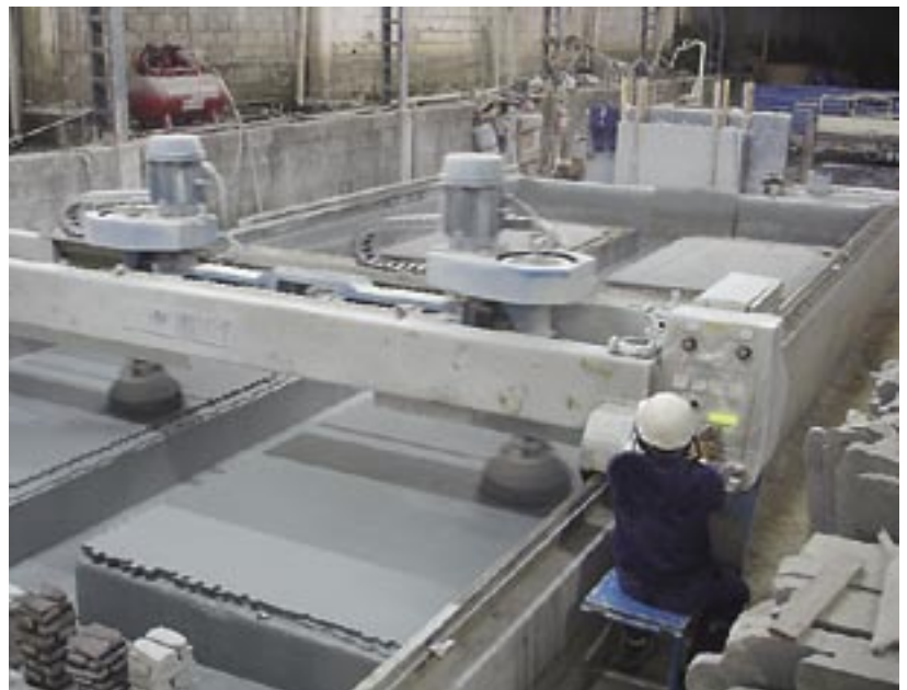
Automatic milling machines hones the plates
